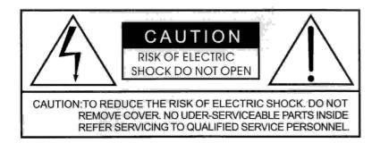
The lighting flash with arrowhead symbol, within an equilateral triangle, is intended to alert the user to the presence of uninsulated." dangerous voltage" within the product's enclosure that may be sufficient magnitude to constitute a risk of electric shock to persons.
