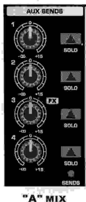
Fig. 2.7: The AUX SEND controls of the main section!
